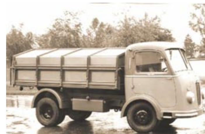
Beta 'cassone chiuso' this one used for transporting grain. The trafficators behind the side window identify it as a pre-1956 model
